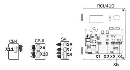
Fig. 20 Terminal diagrams for different cabling variants
