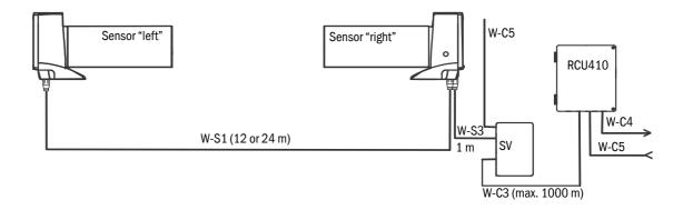
Fig. 17 Variant 5 Additional power supply on terminal boxes on both sensors
