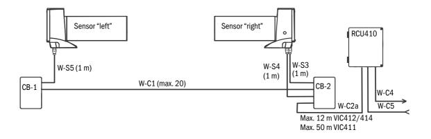
Fig. 15 Variant 3: Terminal box on sensor "right"
